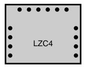
The LZC-4 photoreactor is equipped with 6 top lamps, and 8 side lamps, controlled by 4 switches.
