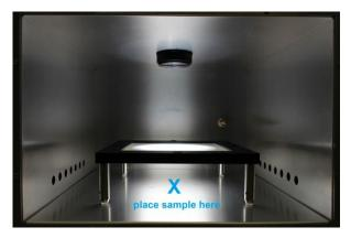
The CCP-SolSim uses a Xenon lamp installed in the tower at the top of the photoreactor chamber, with a custom filter assembly mounted in the chamber ceiling. A proprietary solar simulating filter-diffuser stand with 2" posts is placed on the chamber floor, with samples beneath.
