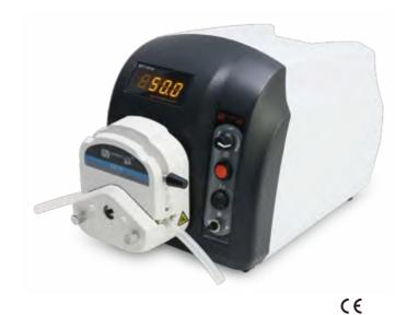
This series of peristaltic pumps use imported core processor, speed control, stepper motor drive, digital display. It has basic functions such an reversible direction, start/stop, full speed (fast cleaning, empty), and speed-variable. Easy dispensing function can realize the repeat timing quantitative dispensing. RS485 interface, as adopting the MODBUS communication protocol, the pump is easier to be connected with other equipments, such as computer, human machine interface and PLC.
