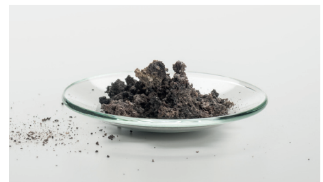
X-ray fluorescence analysis of chimney ash. In the course of its life, the beech wood has not only enriched potassium and manganese, but also considerable amounts of rubidium and strontium.
