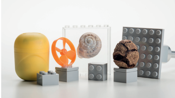
Various objects for a computed tomography, which can simply be attached to the LEGO adapter.
