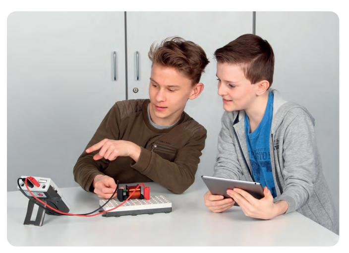
LP3.4.3.1C Electromagnetic induction with bar magnet and a coil
