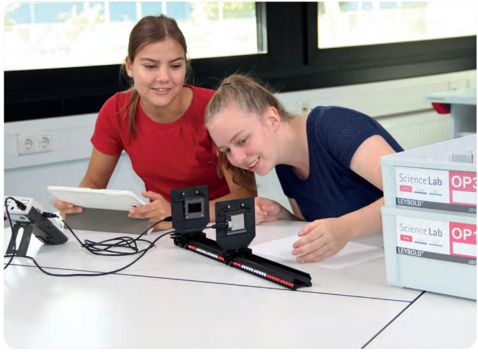
LP5.3.1.1C Diffraction at a slit
