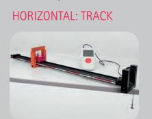
Experiments on uniform and accelerated motion and experiments on collisions
