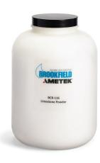
To perform a calibration check on your Powder Flow Tester, use certified BCR-116 limestone powder. Run the standard Flow Function test at 5 consolidation stresses and record the failure strength values. They must be between published min/max values for the instrument to pass. BCR-116 limestone powder is supplied in 3.2kg jars and certified by the European Commission, Community Bureau of Reference. Contact AMETEK Brookfield for more information.
