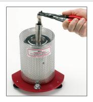
Extracting Tool enables the sample chamber to be handled easily and safely.
