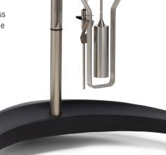
Analyze characteristics such as yield stress, flow curves (mixing, pumping, spraying), leveling and recovery
