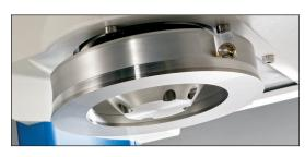
Close-up View of Wall Friction Lid for wall friction and bulk density test
