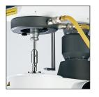
The optional KE cooling device is required to cool viscometer bearings when testing with temperatures above 70°C.
