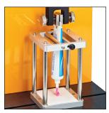
**TA-TEF** *Tube Extrusion Fixture*
