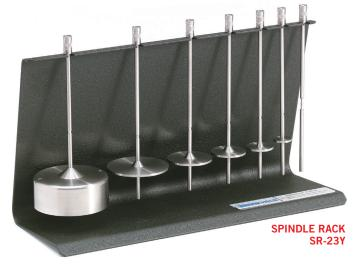
$\mbox{RV/HA/HB}$  Spindle Set includes spindles  $\mbox{\#2}$  -  $\mbox{\#7}$  and is supplied with standard AMETEK Brookfield Viscometers and Rheometers.
