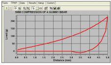
On Screen Live Force Deformation Curve
