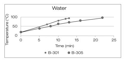
$\Delta T_{_{70\,^{\circ}C\,(water)}}\colon$  B-301 -> 13 min; B-305 -> 22 min
