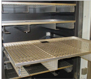
Telescopic rails for simpler loading of the chamber
