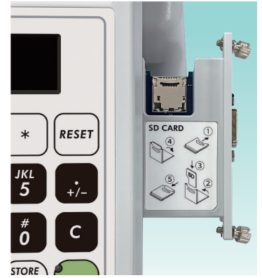
Slot for a MicroSD card
